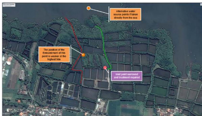
Figure 4. The substitute selection of inlet and outlet alternatives. (Source: Google Earth Image ©2017 CNES/Airbus)
