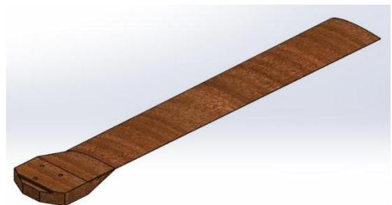
Fig 3. Desain Blade Tapperless 3D NACA 4412.
